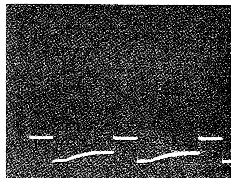
W15 Z112 PIN 10 0.2 V/cm 1 ms/cm DC COUPLED S101 REMOVED TP106 CONNECTED TO TP112, NO INPUT
